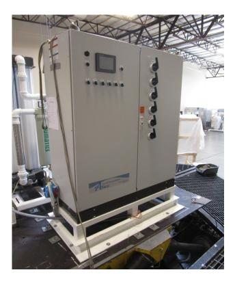
Rigid base mounted: the unit was attached to the shake table with (8) 1/2" diameter Grade 5 bolts.
