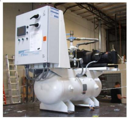
Flexible base mounted: the unit was attached to the shake table with (4) 1/2" diameter Grade 5 bolts, 3/16" thick 4"x4" carbon steel plate, and 4"x4" combination cork and neoprene isolation pads by Vibration Isolation Co., Inc., Model CNP-16.
