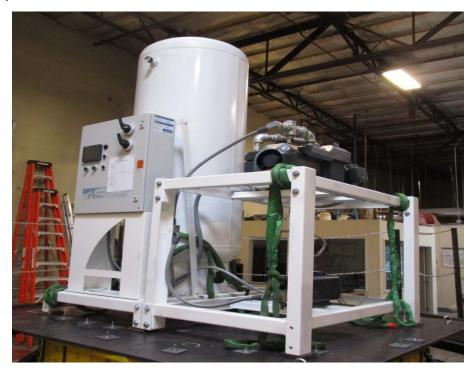
Flexible base mounted: the unit was attached to the shake table with (8) 1/2" diameter Grade 5 bolts, 3/16" thick 4"x4" carbon steel plate, and 4"x4" combination cork and neoprene isolation pads by Vibration Isolation Co., Inc., Model CNP-16.
