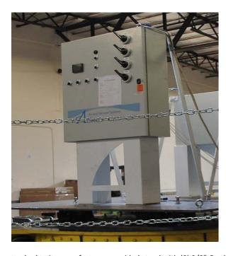
Flexible base mounted: the unit was attached to its manufacturer-provided stand with (8) 3/8" Grade 5 bolts. The stand was mounted to the shake table interface plate with (8) 3/8" diameter Grade 5 bolts. The unit's seismic bracing was attached to the enclosure and to the shake table interface plate with (2) each 3/8" Grade 5 bolts. Interface plate mounted to shake table surface with (4) VMC MSSH-1E-2000 spring mounts.
