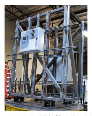
Flexible wall mounted: the unit was attached to the test wall with (4) 3/8" Grade 5 bolts at the back of the enclosure. The test wall was mounted to the shake table with (4) VMC MSSH-1E-2000 spring mounts.
