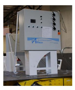
Rigid base mounted: the unit was attached to its manufacturer-provided stand with (8) 3/8" Grade 5 bolts. The stand was mounted to the shake table interface plate with (8) 3/8" diameter Grade 5 bolts. The unit's seismic bracing was attached to the enclosure and to the shake table interface plate with (2) each 3/8" Grade 5 bolts.
