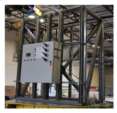
Rigid wall mounted: the unit was attached to the test wall with (4) 3/8" Grade 5 bolts at the back of the enclosure. The test wall was rigidly mounted to the shake table.
