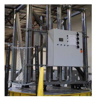
Flexible wall mounted: the unit was attached to the test wall with (4) 3/8" Grade 5 bolts at the back of the enclosure. The test wall was mounted to the shake table with (4) VMC MSSH-1E-2000 spring mounts.
