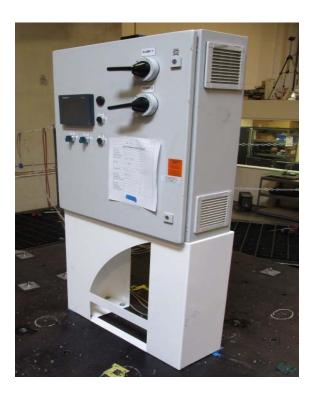
Rigid base mounted: the unit was attached to the manufacturer-provided stand (Amico Part Number STEEL-PDL-APANEL) with (8) 3/8" diameter Grade 5 bolts, (4) on each side of the stand. The stand was mounted to the shake table with (8) 3/8" diameter Grade 5 bolts, (4) in each leg.
