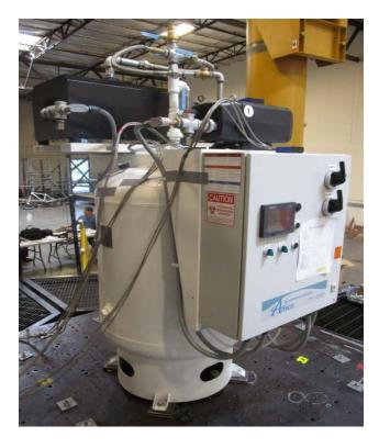
Flexible base mounted: the unit was attached to the shake table with (4) 1/2" diameter Grade 5 bolts, 3/16" thick 4"x4" carbon steel plate, and 4"x4" combination cork and neoprene isolation pads by Vibration Isolation Co., Inc., Model CNP-16.
