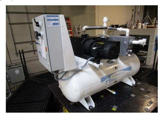
Flexible base mounted: the unit was attached to the shake table with (4) 1/2" diameter Grade 5 bolts, 3/16" thick 4"x4" carbon steel plate, and 4"x4" combination cork and neoprene isolation pads by Vibration Isolation Co., Inc., Model CNP-16.
