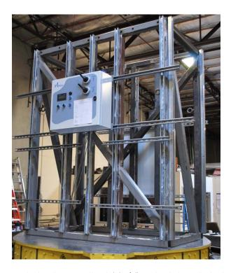
Rigid wall mounted: the unit was attached to the test wall with (4) 3/8" Grade 5 bolts at the back of the enclosure. The test wall was rigidly mounted to the shake table.
