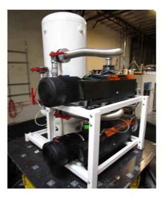
Flexible base mounted: the unit was attached to the shake table with (6) 1/2" diameter Grade 5 bolts, 3/16" thick 4"x4" carbon steel plate, and 4"x4" combination cork and neoprene isolation pads by Vibration Isolation Co., Inc., Model CNP-16. In addition, 1/4" plate washers were added to all receiver tank- to skid mounting locations.
