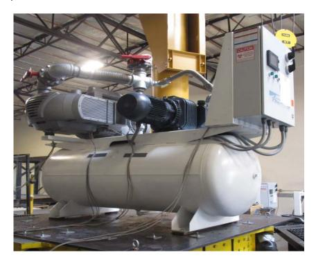
Flexible base mounted: the unit was attached to the shake table with (4) 1/2" diameter Grade 5 bolts, 3/16" thick 4"x4" carbon steel plate, and 4"x4" combination cork and neoprene isolation pads by Vibration Isolation Co., Inc., Model CNP-16.
