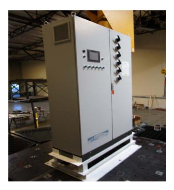
Rigid base mounted: the unit was attached to the manufacturer-provided stand (Amico Part Number STEEL-PDL-REPANEL) with (8) 1/2" diameter Grade 5 bolts (4 at the back and 2 on each side of the unit) The stand was mounted to the shake table with with (10) 1/2" diameter Grade 5 bolts.
