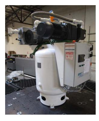
Flexible base mounted: the unit was attached to the shake table with (4) 1/2" diameter Grade 5 bolts, (4) 1/4" thick 2"x2" A36 washers, 3/16" thick 4"x4" carbon steel plate, and 4"x4" combination cork and neoprene isolation pads by Vibration Isolation Co., Inc., Model CNP-16.
