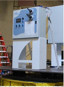
Flexible base mounted: the unit was attached to its manufacturer-provided stand with (6) 3/8" Grade 5 bolts. The stand was mounted to the shake table interface plate with (8) 3/8" diameter Grade 5 bolts. The unit's seismic bracing was attached to the enclosure and to the shake table interface plate with (2) each 3/8" Grade 5 bolts. Interface plate mounted to shake table surface with (4) VMC MSSH-1E-2000 spring mounts
