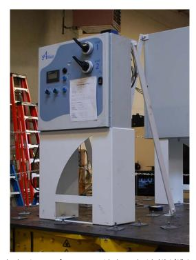
Rigid base mounted: the unit was attached to its manufacturer-provided stand with (6) 3/8" Grade 5 bolts. The stand was mounted to the shake table interface plate with (8) 3/8" diameter Grade 5 bolts. The unit's seismic bracing was attached to the enclosure and to the shake table interface plate with (2) each 3/8" Grade 5 bolts.
