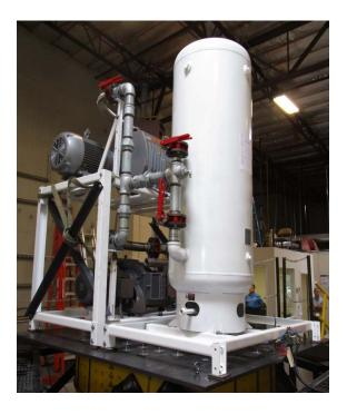
Flexible base mounted: the unit was attached to the shake table with (8) 1/2" diameter Grade 5 bolts, 3/16" thick 4"x4" carbon steel plate, and 4"x4" combination cork and neoprene isolation pads by Vibration Isolation Co., Inc., Model CNP-16. Pre-test retrofit: the pump frame was braced on each short side with two pieces of 2-1/2"x1/4" carbon steel angle, using two of the existing 1/2" diameter Grade 5 frame bolts to attach each angle.
