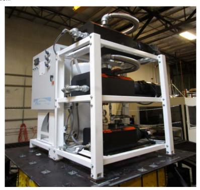
Flexible base mounted: the unit was attached to the shake table with (8) 1/2" diameter Grade 5 bolts, 3/16" thick 4"x4" carbon steel plate, and 4"x4" combination cork and neoprene isolation pads by Vibration Isolation Co., Inc., Model CNP-16. All factory installed pump isolators were replaced with VMC TTB-750 isolators.
