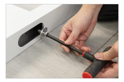
After tightening the 3/8" socket cap screws, position the two posts vertically and place the track assembly at the top of the two posts.
