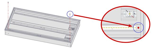
5. Swing open the Eclipse insert and attach the desired conduit to one of the inlet holes #1, #2, or #3.
