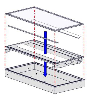
8. Fixture is designed for use with 1.00"/1.50" T bar grid systems with vertical grid T thickness of less than 1/4" with a maximum height of 1.50".
