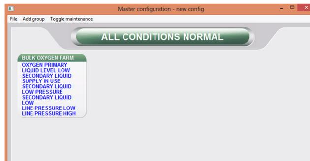
3. Save the Configuration file to the SD Card. The file name must be saved as master.cfg in the “Master Configuration” file type.
