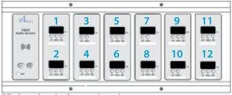
"X" indicates the order of gases, as shown above. example: OAV (position 1 OXY, position 2 AIR, position 3 VAC)
