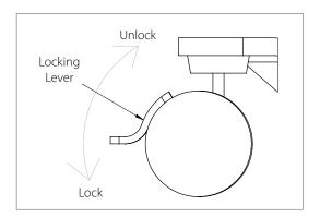
i NOTE: To lock the casters, step on the locking level until it clicks in the down position. To unlock the caster, lift up the locking lever.
